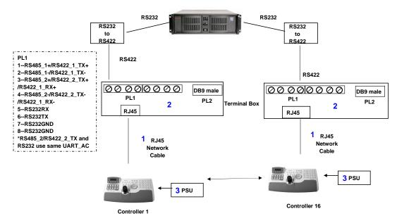
Figure 4-10 RS232 Serial Port Connection, MX18 and the Terminal Box
